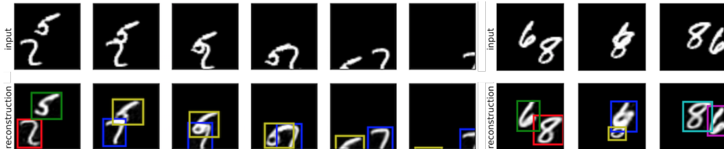
Figure 12: Two failed reconstructions of SQAIR. Left : SQAIR re-detects objects in the second time-step. Instead of 5 and 2, however, it reconstructs them as 6 and 7. Interestingly, reconstructions are consistent through the rest of the sequence. Right : At the second time-step, overlapping 6 and 8 are explained as 6 and a small 0. The model realizes its mistake in the third time-step, re-detects both digits and reconstructs them properly.
