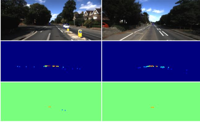
Fig. 4. Examples of automatically generated training data. *Top* shows the image with bounding boxes from the object detections from the combined cameras. *Middle* shows the range image generated from the radar scan and *bottom* shows the range-rate image. Note the difference in colour of the signals associated with the oncoming and retreating vehicles in the left-hand range-rate image. The colouring of the radar images is for visualisation only.
