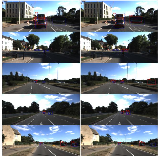
Fig. 11. Comparison of detections using both networks. *Left* are detections from the RGB only network. *Right* are from the network using both RGB and radar. Detections are in red with confidences, automatically generated (and hence imperfect) ground truth in blue.
