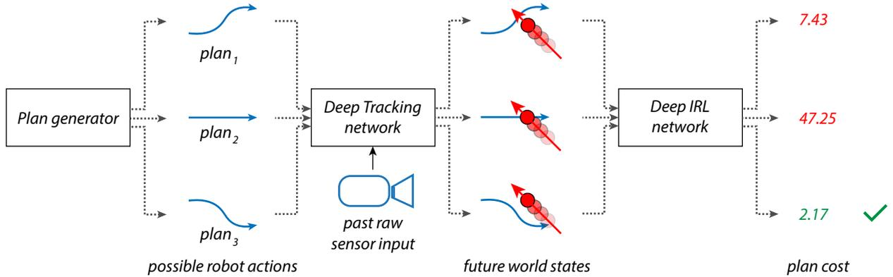
Figure 3: Proposed Neural Robotics pipeline. The Plan Generator synthesises a set of possible plans of actions. Deep Tracking Network acts as an oracle capable of predicting the future world states in response to any given plan of actions. The plan with the lowest cost as evaluated by the Deep Inverse Reinforcement Learning (IRL) network is then selected for execution.
