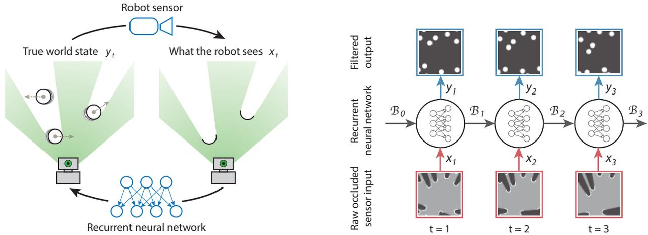
Figure 2: Robot’s sensors provide only partial observations of the surrounding environment. DeepTracking leverages a recurrent neural network to effectively reveal occluded parts of a scene by learning to track objects from raw sensor data – thereby effectively reversing the sensing process.
