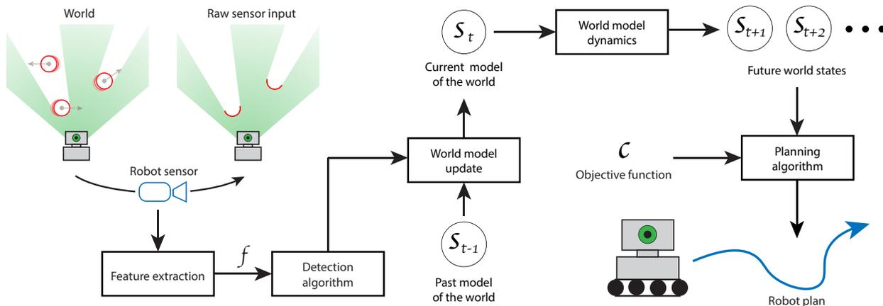
Figure 1: An example of a traditional robotics pipeline. Several hand-designed data processing stages necessary for the operation of the robot result in the sub-optimality of the whole system.
