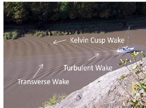
Figure 4: Boat wake components
