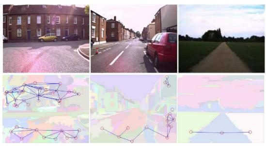
Fig. 5 Typical graphs extracted from urban scenes as recorded by our mobile robot. Top: the original scenes. Bottom: the corresponding segmented images with the extracted graph overlaid. Circles indicate nodes, lines indicate edges. For images patches which are not marked as nodes no reliable geometry estimates could be extracted from the laser data.
