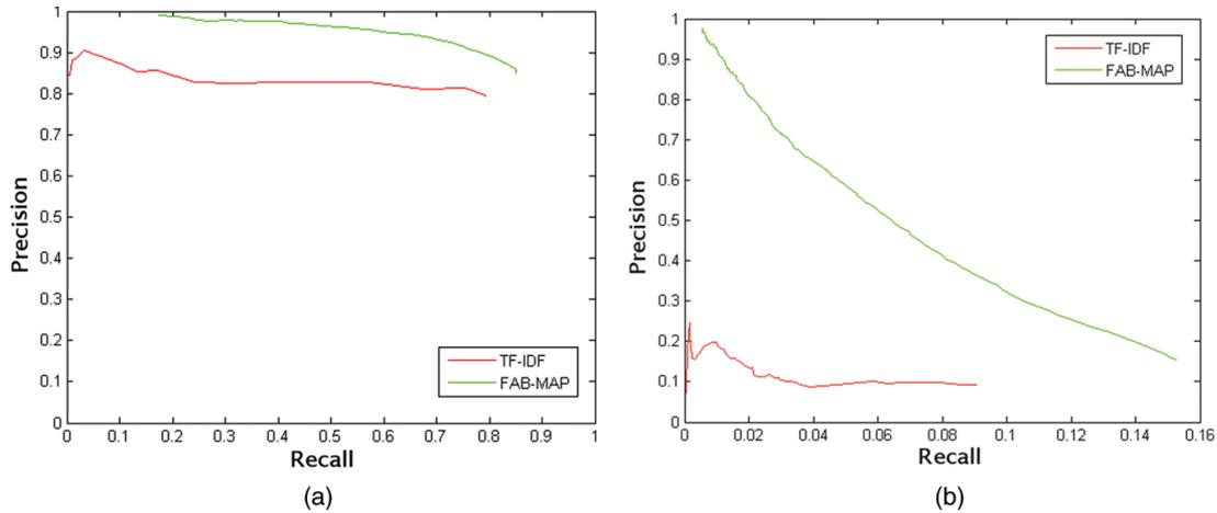
**Fig. 12.** Comparison to tf-idf ranking: (a) 70 km set; (b) 1000 km set. FAB-MAP substantially outperforms this standard ranking metric, particularly on the larger data set. To ensure the fairest possible comparison, these performance figures relate to a retrieval-only task that excluded new place detection. See Section 7.4 for details.
