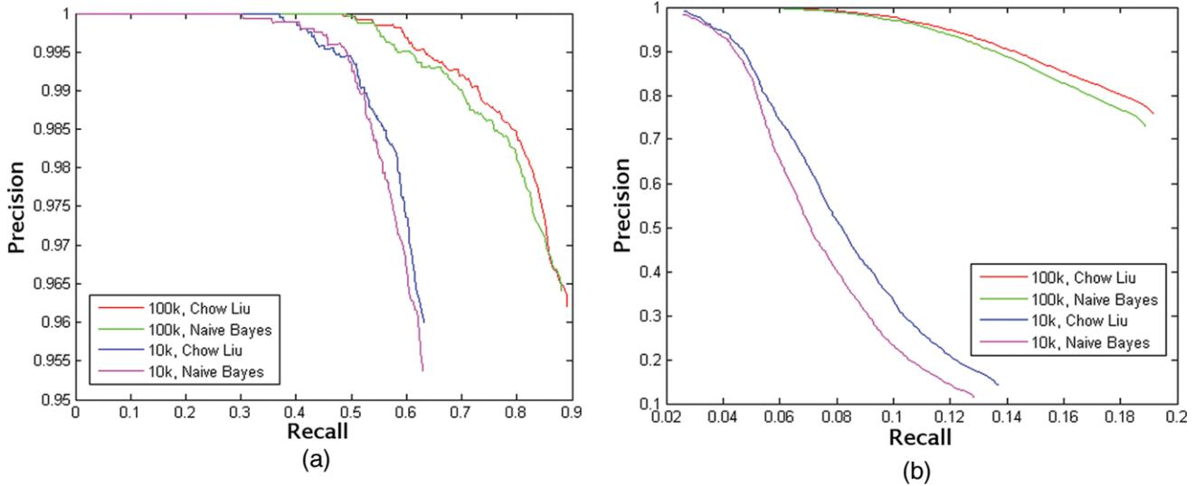
**Fig. 11.** Precision–recall curves showing the effect of the vocabulary size and the Chow Liu tree on performance: (a) 70 km set; (b) 1000 km set. Note the scaling on the axes. Performance shown includes motion model and geometric check. Performance increases strongly with vocabulary size. The Chow Liu tree also increases performance, for all vocabulary sizes.
