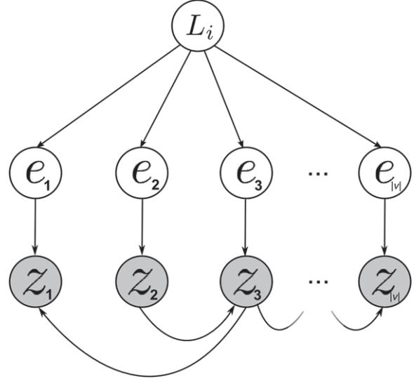
**Fig. 2.** Graphical model of the system. Locations  $L_i$  independently generate scene elements  $e_q$ . Visual word detections  $z_q$  are conditioned on scene elements  $e_q$  via the detector model, and on each other via the Chow Liu tree.
