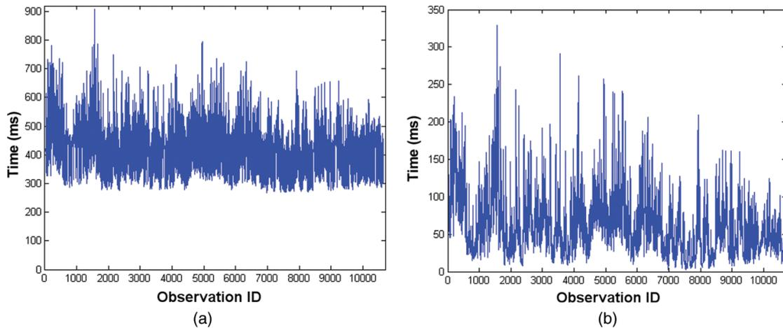
**Fig. 13.** Bag-of-words generation time (per Ladybug2 panoramic image) for a representative sample of the 1000 km data set, using the 100k vocabulary. The time is dominated by SURF generation, (a), which takes 423 ms on average. Quantization using the randomized kd-trees, (b), takes on average 60 ms.
