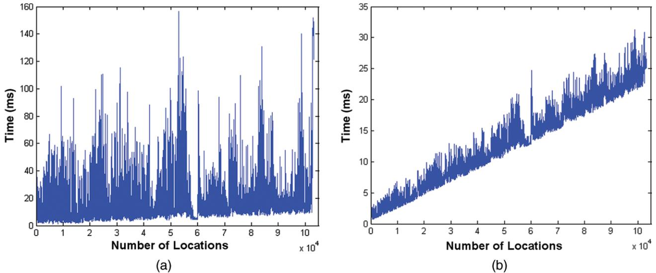
**Fig. 14.** Filter update times on the 1,000 km data set for the 100k vocabulary, (a). Mean filter update time is 14 ms and maximum update time is 157 ms. The cost is dominated by the RANSAC geometric verification, which has  $O(1)$  complexity. The core ranking stage excluding RANSAC, (b), exhibits linear complexity but with a very small constant - taking 25ms on average with 100,000 locations in the map.
