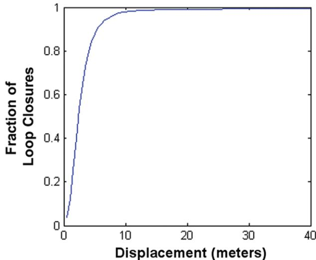
**Fig. 9.** The typical displacement in meters between two images identified as loop closures. While any pair separated by less than 40 m is accepted as a true positive, because the ground truth separation can occasionally be this large, 89% of detected loop closures are separated by less than 5 m, and 98% by less than 10 m.
