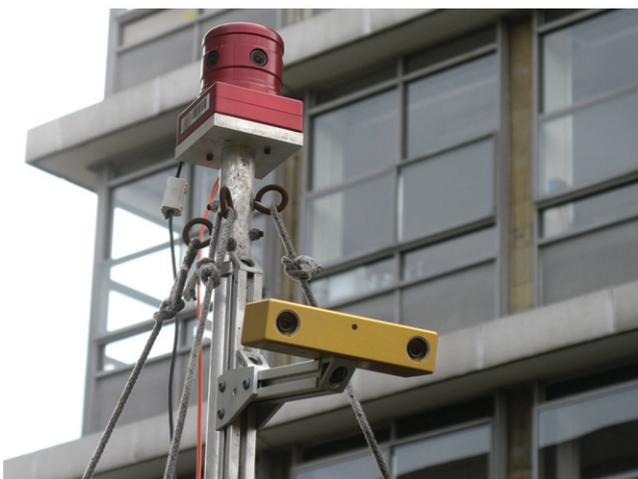
**Fig. 8.** Vehicle and sensor rig used to capture the 70 km and 1000 km data sets. The rig consists of a Ladybug2 omnidirectional camera and Bumblebee stereo camera, both from Point Grey Research. The cameras were mounted approximately 3 m above the road surface. GPS data was collected with a Seres unit from CSI Wireless, mounted on the roof of the car.
