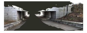
Fig. 5. An example dense reconstruction produced by fusing laser data into a voxel grid and applying texture to the surfaces from camera data.
