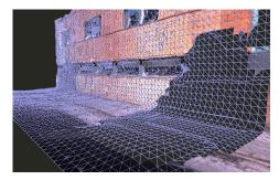
(a) The raw pointcloud used as the input to our regularisation algorithm.
