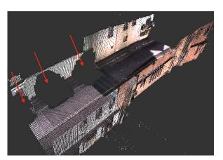
(a) Before: The *sparse* laser point cloud input after removing ephemeral objects (automobiles). The resulting gaps are highlighted by red arrows.
