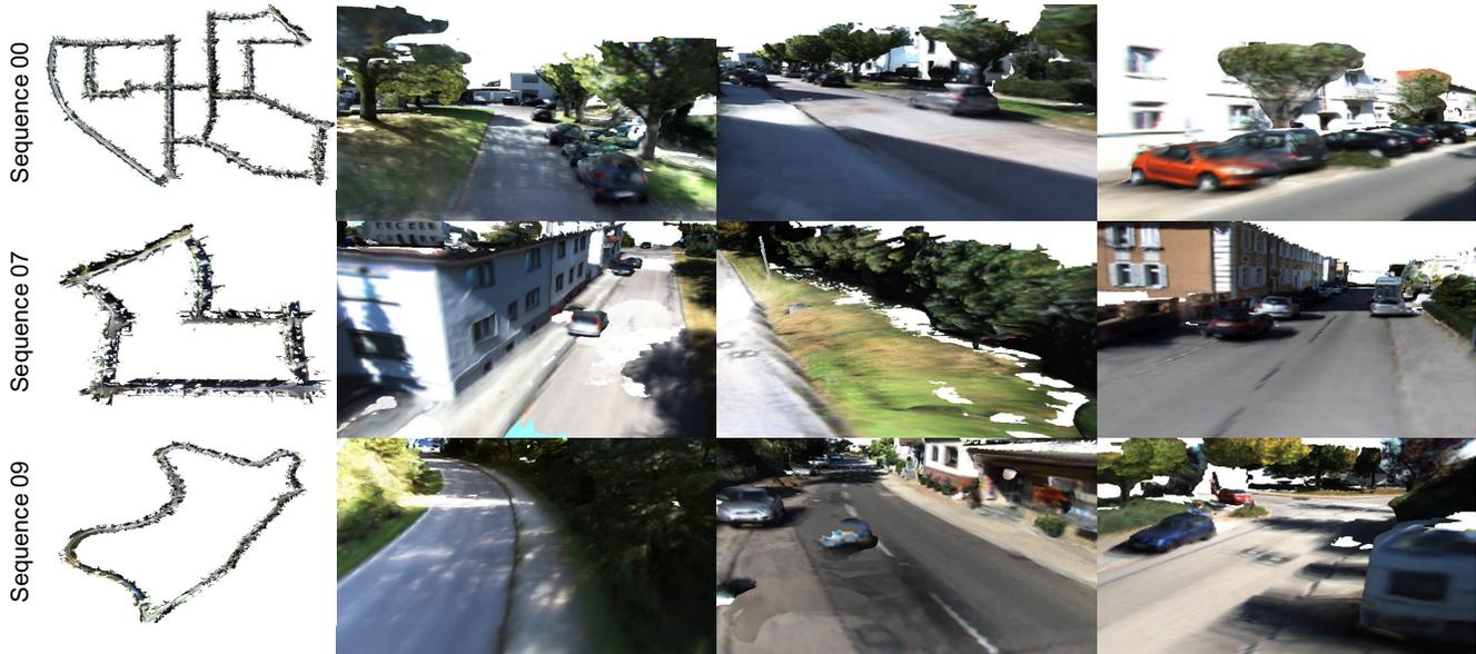
Fig. 6. A few representative sample images for various points of views (offset from the original camera’s position) along each trajectory. All sample images are of the final regularized reconstruction with 10 cm voxels. The video provides full fly-through footage for each sequence.
