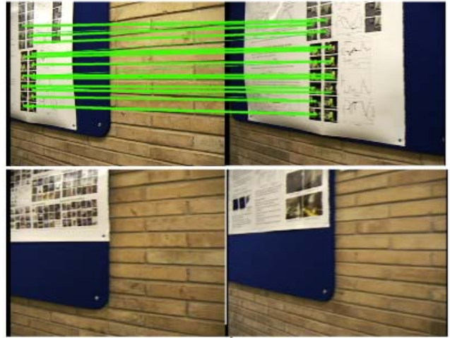
Fig. 5. View of the feature to feature correspondences found between the two images (top right and top left) used in the loop closing event shown in figure 3. The lower two images show similar images in the database that were successfully discriminated against.
