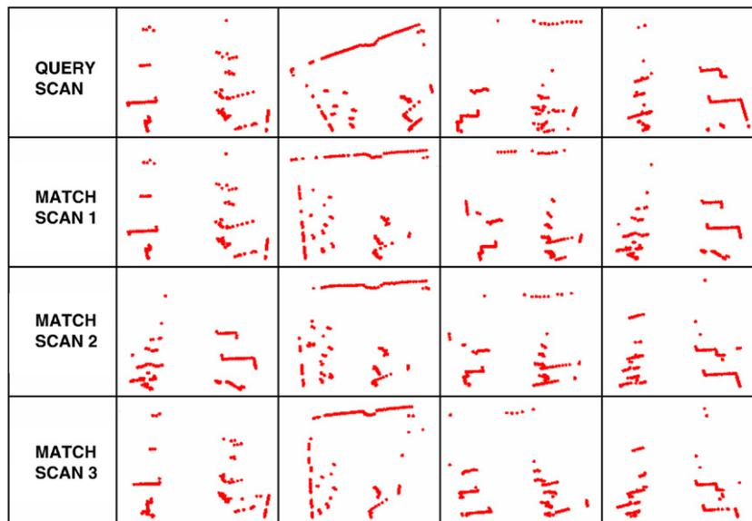
Fig. 10. Experimental results from our laser scan shape-based query system. The top row contains the query laser scans. Down the column are the corresponding matches in descending order of similarity.
