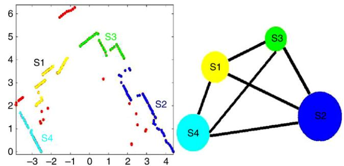
Fig. 4. This shows a typical geometry patch after segmentation and a graph depiction of the way we encapsulate the information contained. Each node is a segment and contains the CAF function, its entropy measure and a list of critical points. The edges represent a known spatial relationship between segments.
