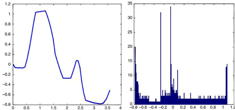
Fig. 5. The cumulative angular function is transformed into a histogram of angular values. Each bin contains the number of points along the cumulative angular function that have angular values that fall within the bin value. Using this histogram of bin values, the entropy of the cumulative angular function can be calculated.
