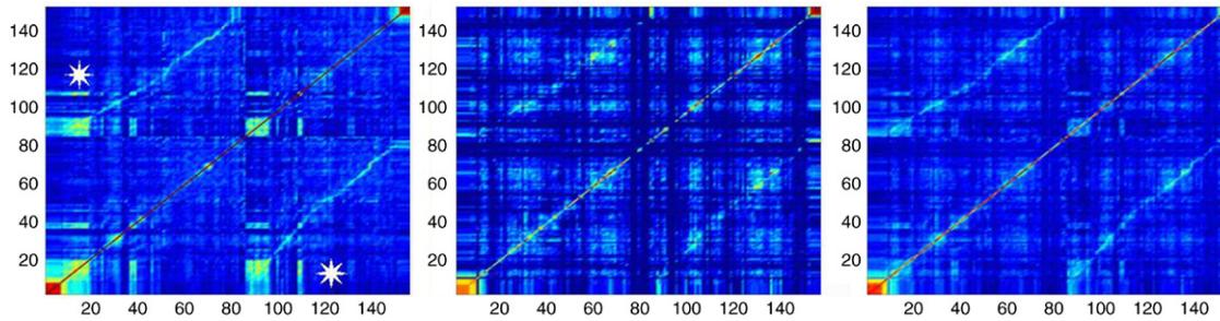
Fig. 11. Similarity matrices. The left matrix is the image similarity matrix. The middle matrix is the laser scan similarity matrix. The right matrix is the combined image–laser scan pair similarity matrix. Improvement in loop closure detection can be observed by the improved definition of the off-diagonals of the combined image and laser scan pair similarity matrix over the off-diagonals of the other similarity matrices.
