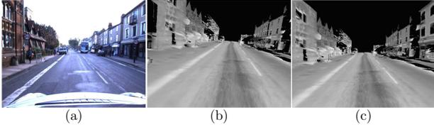
Figure 4. Camera-LIDAR calibration rendered using LIDAR reflectance information. (a) shows the reference camera image, and (b) the resulting scene prior with a calibration estimate with an orientation error less than 10 degrees. (c) shows the correct calibration recovered by the NID minimisation over a series of ten images.
