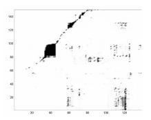
Fig. 7. A visual similarity matrix constructed from the union of two image sequences collected by two robots (before rank reduction). The maximally aligned sequence allows detection of the intersection of the scenes experienced by the independent robots and unification into a common co-ordinate frame.
