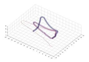
Fig. 6. Vehicle poses prior to any loop closure are shown as a thin line. Small spheres indicate rigid groups of poses whose inter-frame transformations are optimised. The open loop is the result of attempting to apply a lop closure constraint in one step while the closed loop results from iterative non-linear optimisation.
