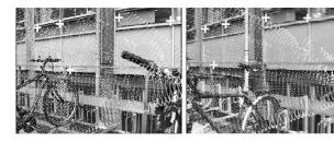
Fig. 5. Calculating the loop closure geometry. Using five or more correspondences (crosses) between Harris Affine features, the transformation between two views can be deduced up to scale. 3D laser data is back projected onto the images (white dots) to find the range of the interest points and thus remove the scale ambiguity. The distribution of laser points is due to the combination of vehicle motion and "nodding" motion of the laser scanner.
