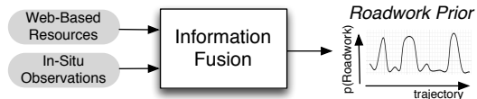
Fig. 1. Data fusion of web-based resources (e.g. websites citing the expected locations of roadworks) and in-situ observations (detections of roadwork indicators as in Fig 2) to estimate a roadwork prior.
