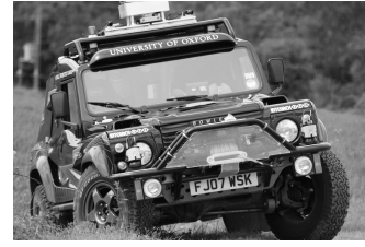
Fig. 3. The Wildcat autonomous car, pictured above, was used to collect the data used in this paper. It is equipped with a Bumblebee stereo camera, capturing 512x384 colour images at 20Hz and a differential GPS/IMU which we use for localizing city council observations along the vehicle's trajectory. Data was collected over a period of 3 months. In this paper, we process 38.98GB of data.
