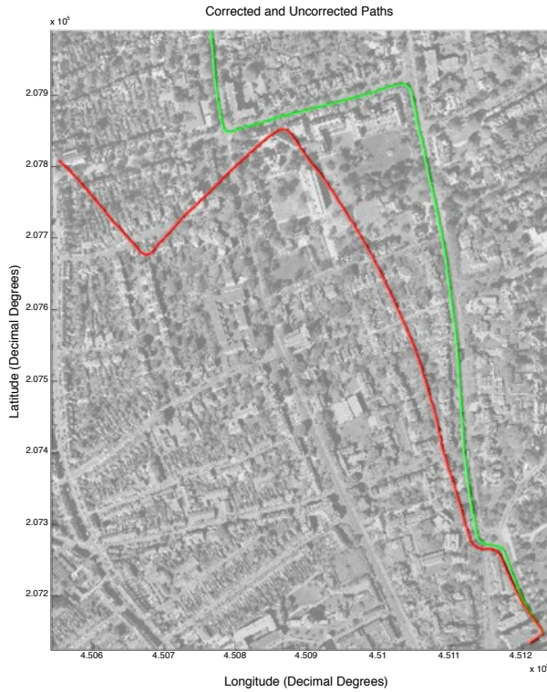
Figure 5: Part of the 100km Highway dataset RBA (red) and corrected onto the road (green).
