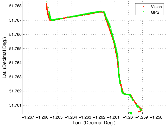
Figure 8: GPS vs visual path estimate for the start of the Highway data. Error in latitude and longitude are shown in Figures 9 and 10.
