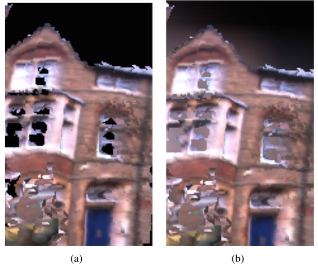
Fig. 4. We render our synthetic images at two resolutions, and use the lower resolution version to fill in gaps in the higher resolution image. This prevents sharp changes at the edges of the mesh from dominating image derivatives. (a) A segment of the higher resolution image. (b) The same image filled in with a slightly lower resolution image, producing blurring around edges and filled-in holes in the windows.
