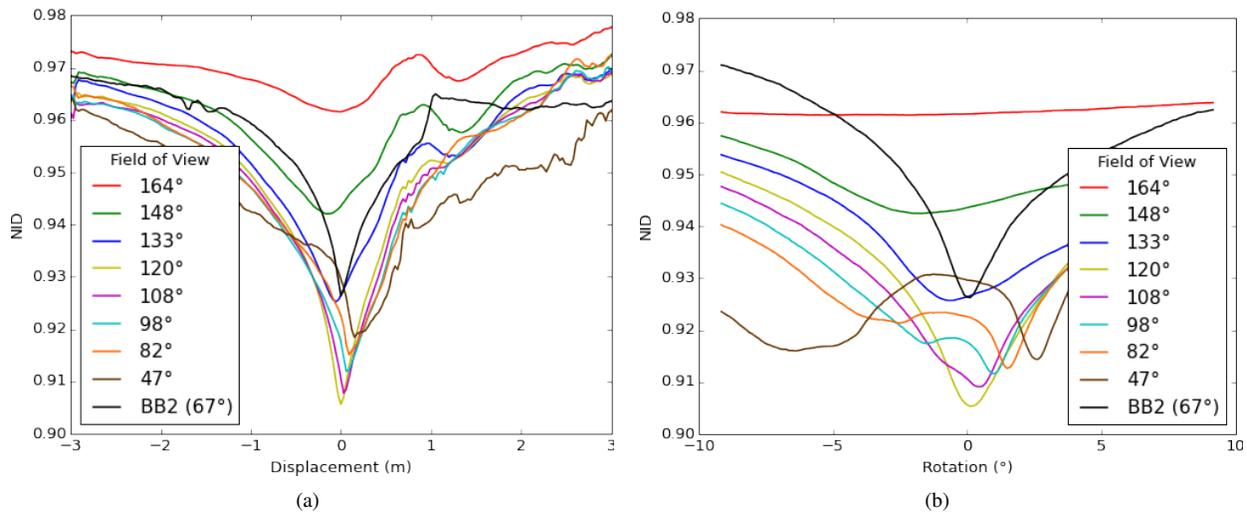
Fig. 10. NID curves with varying fields of view. Each curve is the mean of the three translational or rotational axes, averaged across 20 locations.
