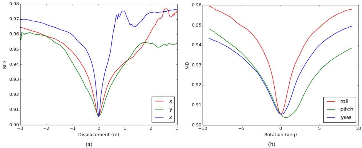
Fig. 8. NID values at varying offsets from the ground truth pose. These plots are averaged across 20 different locations. (a) Translational axes with  $x$ ,  $y$  and  $z$  shown as red, green and blue respectively. (b) Rotational axes with roll, pitch and yaw shown as red, green and blue respectively. The second local minimum in the  $z$  axis is due to the road looking very similar when rendered from below as it does from above.
