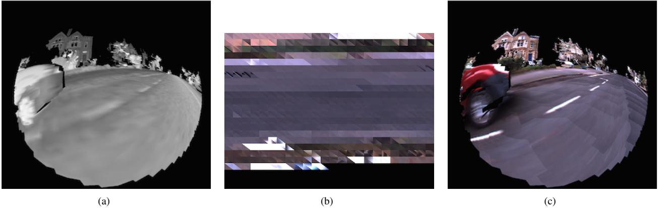
Fig. 2. Generation of the prior: (a) First we build a mesh by stitching together subsequent scans from the push-broom LIDAR; (b) we then project the mesh in turn into each camera image, and generate a texture for each triangle — here we show all the textures for a single ‘slice,’ from many different input images; and (c) we combine all the slices with their textures for the final prior.
