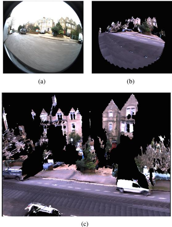
Fig. 1. Our localisation system relies on generating virtual images from a map consisting of a textured mesh, and comparing those images with the live camera feed. We use a simple look-up-table based distortion model to create virtual images with the same distortion as the live camera lens. (a) Live camera image, (b) projection of the prior using a highly distorted model, (c) a birds-eye view of the prior at the same location.
