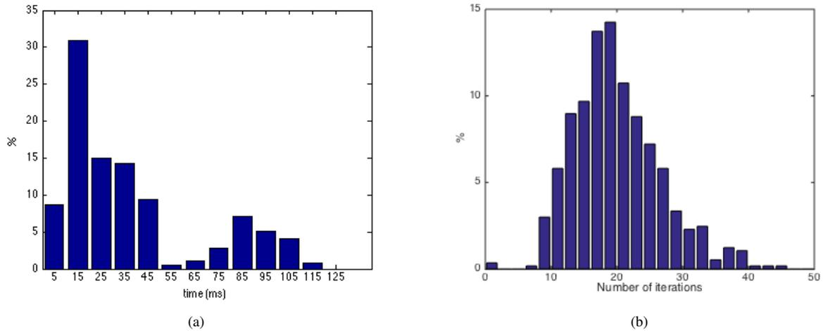
Fig. 9. Runtime behaviour of optimiser. (a) Time taken to evaluate the NID function, including rendering the synthetic image. The majority of cost function evaluations take less than 25 ms. (b) Number of cost function evaluations carried out in each optimisation. Most optimisations require approximately 20 evaluations.
