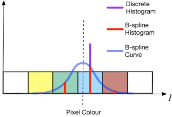
Fig. 3. Building a differentiable histogram. Rather than incrementing only the bin into which a pixel value falls, we add the coefficients from a cubic B-spline using supports at the centre of each bin. Because the histogram values now depend not only on which bin a pixel falls into, but *where* in that bin the pixel falls, the histogram becomes a continuous function of the pixel values. This diagram shows the effect of adding a single pixel to the histogram.
