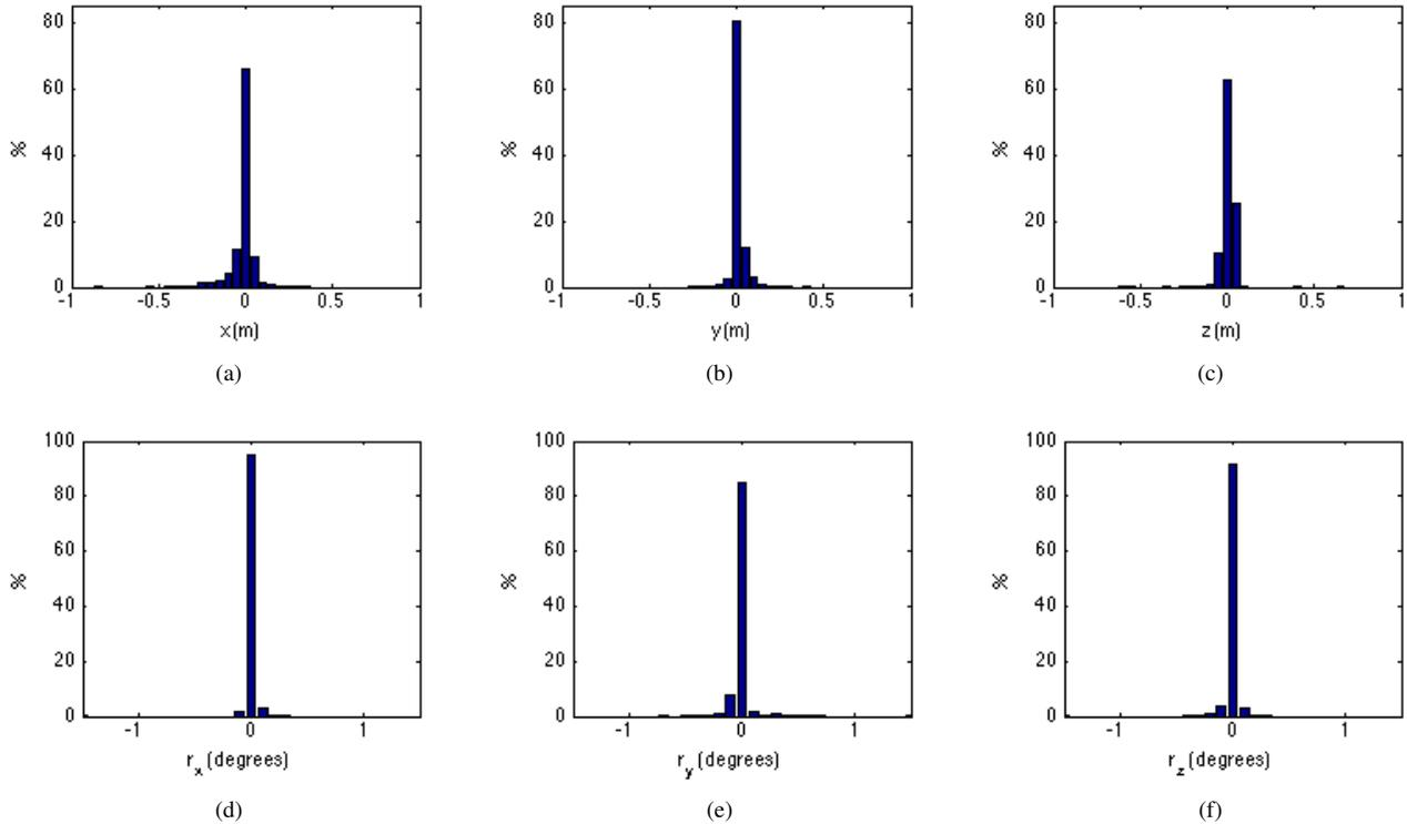
Fig. 7. Histograms showing displacement between the localised solution and ground truth in each degree of freedom. The coordinate system places  $x$  in the direction of the vehicle’s travel,  $y$  to the vehicle’s right, and  $z$  downwards into the road.
