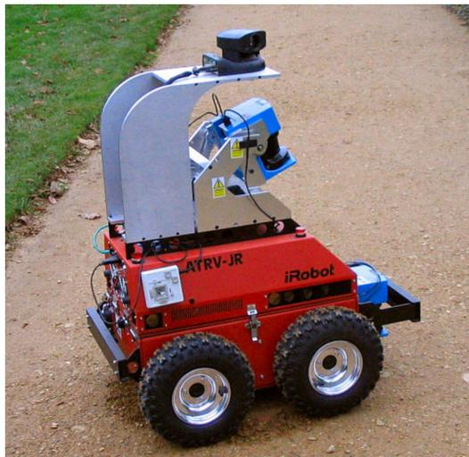
Fig. 1. Our 3D scanning laser range finder mounted on research vehicle ‘Marge’.
