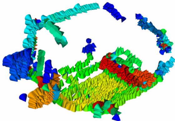
Fig. 4. The result of applying the normal estimation process to the scene shown in Figure 2. The coloring indicates the traversal order of the MST from red to blue.
