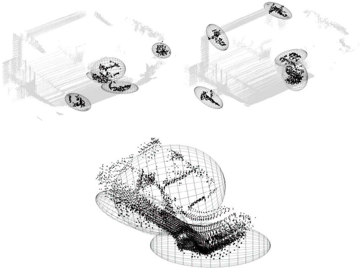
Fig. 6. The same data as shown in Figure 2 but with the top five salient regions highlighted in each case. Note how the shape of the car is categorized as salient along with the multifaceted corners of the overhead concrete gantry. The ellipsoids are for illustrative purposes only and are scaled covariance ellipsoids of the raw data points which constitute each of the salient regions. They serve to illustrate their crude shape and location.
