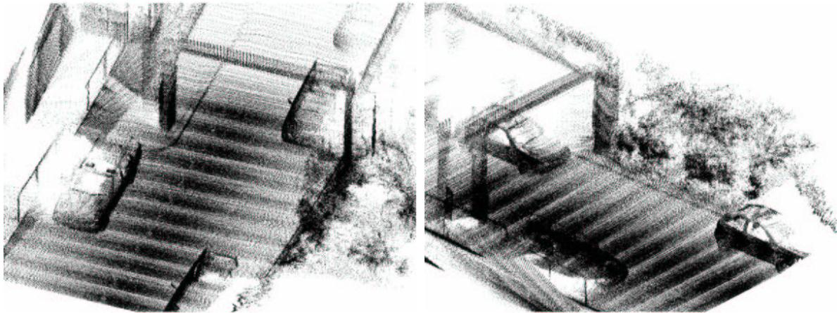
Fig. 8. A short dose of SLAM using sequential registration of 6 D.O.F. pose states. The above figure is generated by sequentially registering the salient regions from twelve 3D scan patches captured at 1m intervals. The entirety of each scan patch is rendered from the corrected vehicle position.
