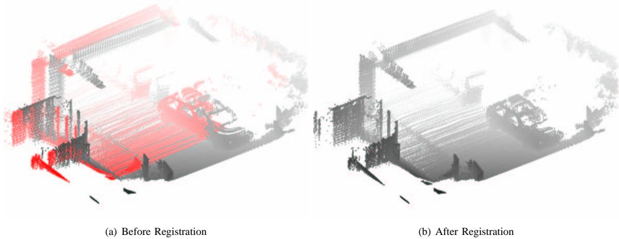
Fig. 7. Registration using salient regions. The salient regions of Figure 6 are registered using the method described in Section V. To illustrate the problem, the left hand Figure shows two data sets with an artificially elevated relative orientation and translational error. The right hand figure shows the same two data sets after registration. Note how the use of a robust kernel (e.g Huber or Cauchy) means that we do not require the same number of data points or clusters in each patch.
