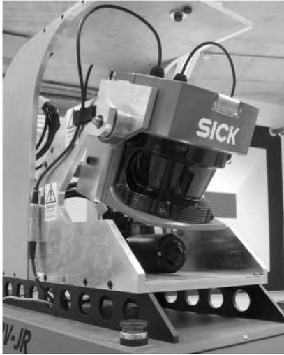
Fig. 1. The nodding 3D laser range finder mounted on a mobile robot
