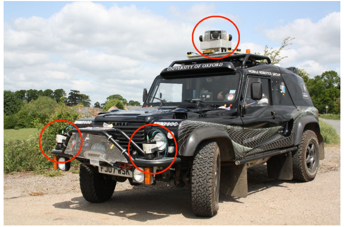
Figure 2: The Wildcat vehicle has a spinning 3D LIDAR on the roof, and two 2D LIDARs on the front bumper at different elevation angles (sensors circled in red). The INS system is mounted over the rear axle.
