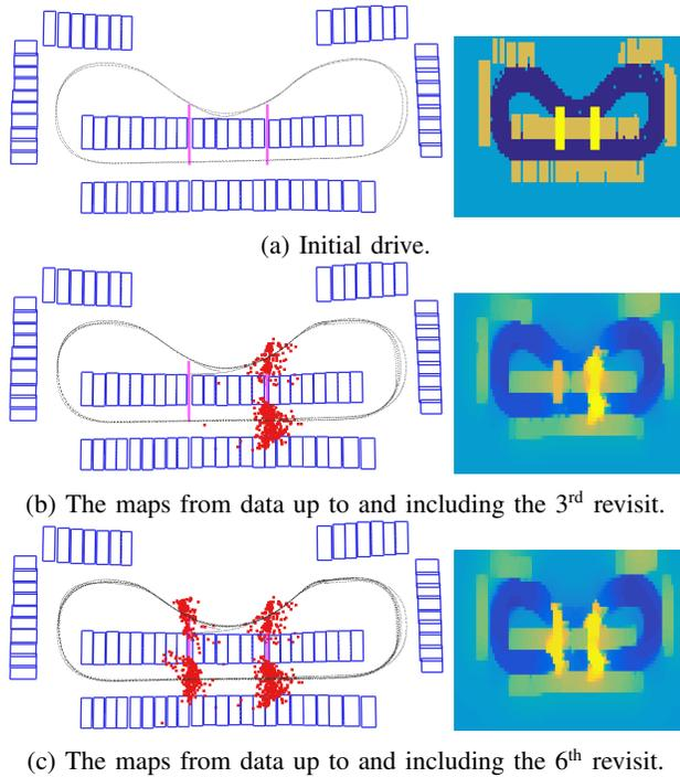
Fig. 10: On the left, the red dots represent projections of the detected pedestrians into the static map. On the right, the evolution of the dynamic map as more pedestrians are detected. In the dynamic map, blue represents lower danger (higher speed) and yellow represents more danger (higher speed). The top dynamic map is calculated using only the prior over pedestrians given the static map.
