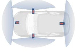
Fig. 4: The configuration of the four 180° field-of-view fish-eye cameras used for mapping, localisation, and dynamic object detection.
