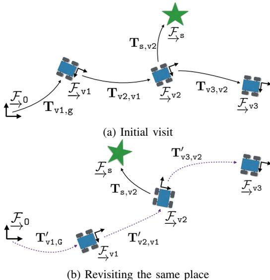
Fig. 3: While the vehicle positions  $[v_1, v_2, v_3]$  may be recomputed between (a) the initial visit and (b) the revisit, the position of the semantic object  $s$  relative to  $v_2$  remains unchanged. This allows us to update the metric map without having to recreate the semantic labels.  $\mathcal{F}_0$  represents the global origin coordinate frame, and  $T_{a,b}$  represents a 6 d.o.f. transformation from  $b$  to  $a$ .
