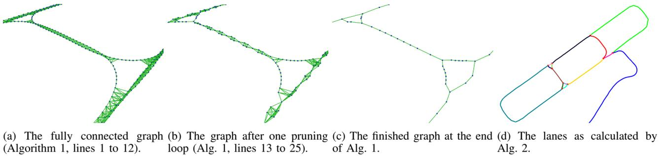
Fig. 8: The process of calculating the road network using the method from Sec. V-B applied to the Stuttgart car park.
