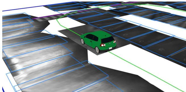
Fig. 1: The semantic information placed relative to the metric map. Shown are the driving lanes in green, and the parking spaces in blue.
