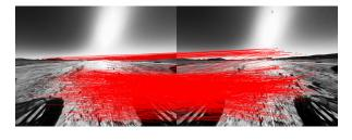
Figure 6. Sample imagery showing interesting features (detected and described by SURF) on two subsequent images captured by the rover as it moves, and matches from frame-to-frame
