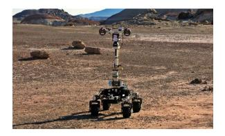
Figure 1. The Q14 Rover and PANCAM emulator. The PanCam is mounted at the top of the mast and can be rotated through 360 degrees and angled up/down using a mast mounted pan/tilt unit. The XB3 is the gold unit half way up the mast, the LIDAR is just below, and and the Grasshopper is mounted on the front of the rover platform bed.
