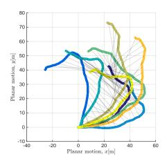
Figure 8. The gray lines connecting these colourful traces indicate the localisation of one drive (experience) to another. The frequency of these connecting lines increases with the accuracy of the metric pose estimate relative to the corresponding experience. This shows that despite accumulating error in the global position of the robot, it can still reliably localise (enabling accurate control), aided by a constantly evolving representation of the world.
