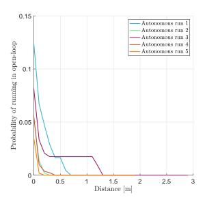
Figure 5. Probability of running without localisation (in open-loop mode) for the simulated autonomous runs. The horizontal axis represents the distance travelled in open-loop. The vertical axis represents the probability of travelling a certain distance in open-loop mode.
