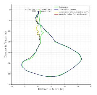
Figure 3. Path driven by the rover during the first simulated autonomous run, with the experience map in green, and the first simulated autonomous run in yellow, blue and red.
