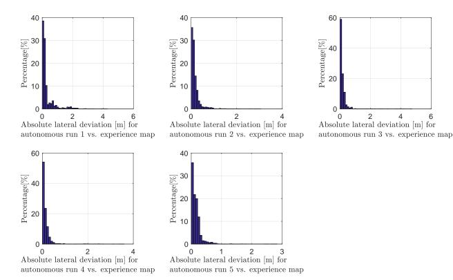
Figure 4. Lateral deviation histograms of the simulated autonomous runs from the reference experience map (not cumulative). The horizontal axis represents the lateral deviation in metres. These results show that Dub4 is capable of closely following the experience map, with most deviations within 0.5m.
