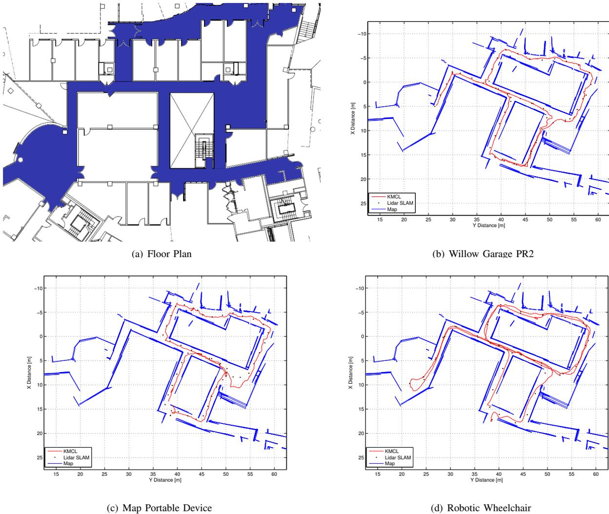
Fig. 8. Top-down view of mapping performance for three of the robots localizing using the same map (non-simultaneously). The main walls in the map are shown in blue while each robot’s Kinect MCL output is shown with a red line. Black dots indicate the ground truth position during the runs (estimated using LIDAR SLAM) — which indicates accurate localization.
