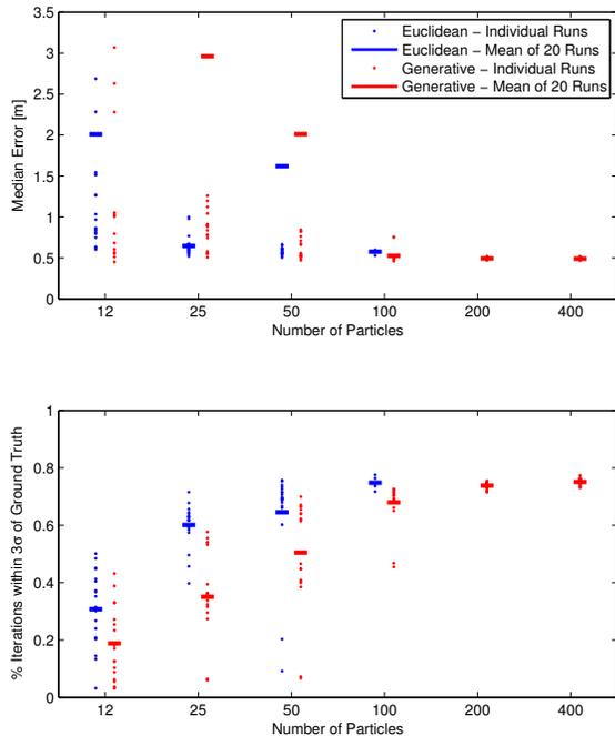
Fig. 9. Performance metrics for both likelihood functions (averaged for 20 separate runs). Typical performance for 100 particles is of the order of 0.5 m median error and 78% of estimates within  $3\sigma$  of the true location. Note that for some failed runs with low particle numbers the median error is greater than 3.5m.
