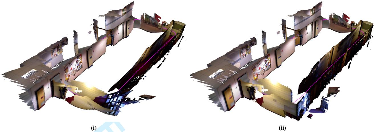
**Figure 12:** From left to right; (i) Highly distorted map produced when a naive nearest neighbour sampling and connectivity strategy is used; (ii) Non-distorted map loop closure using our proposed sampling and connectivity strategy.
