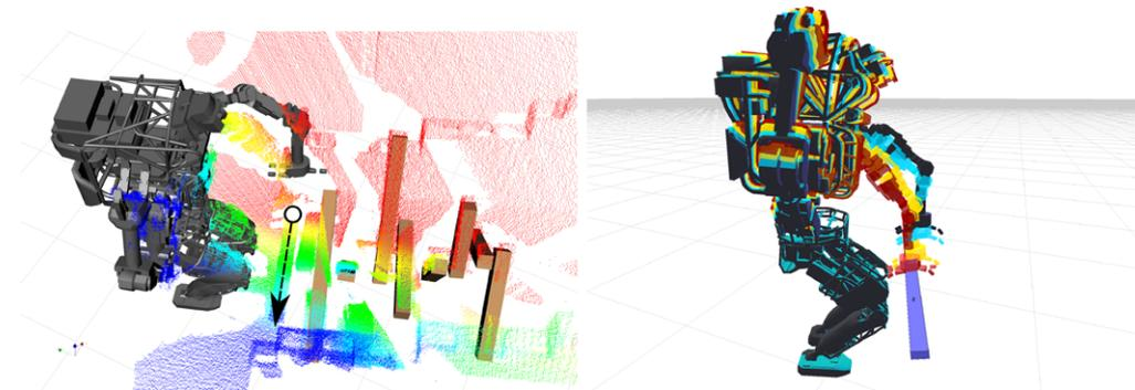
**Figure 12.** A fitting algorithm produces an affordance that can be used to plan a reach motion. Left: A line annotation (arrow) defines a search region that is used by a segmentation algorithm to fit a 2 in.  $\times$  4 in. board affordance to the 3D point cloud data. Right: An end effector goal placed on the board affordance is used to compute a reaching plan.
