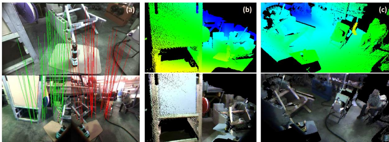
**Figure 5.** Chest camera alignment. (a) SIFT feature matches extracted between head image (top) and left/right chest camera images (bottom) used to align the sensor frames. (b,c) LIDAR points pseudo-colored by distance (top) and texture-mapped with chest camera images (bottom), demonstrating accurate alignment between head and chest data.
