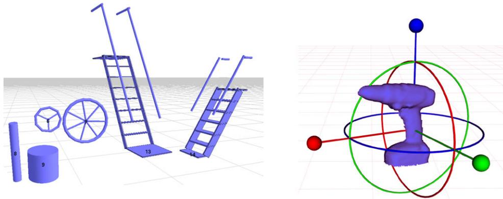
**Figure 11.** Affordances were represented in a parametrized XML format. Left: a collection of objects under three templates: (i) cylinder; (ii) valve; and (iii) angled ladder. Two pairs of objects are shown under each affordance class, which are instantiations with different parameters. Right: Interactive markers allowed the user to adjust the position of an affordance, or to instruct the robot to move the affordance along one of its internal degree of freedom.
