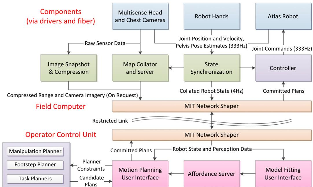
**Figure 6.** The major software components of our system. A series of processes running on the robot collated kinematic and perception sensor data, and responded to operator requests for LIDAR and imagery (green). The operators interpreted this data (pink) and formulated motion plans (purple), which were executed by the robot controller (purple). Data was transmitted across DARPA’s restricted link by our network shaper software (orange).
