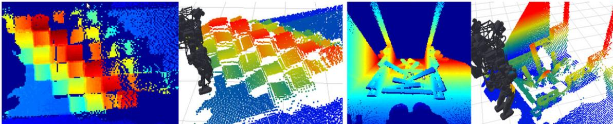
**Figure 7.** Sample composite views of raw laser range data. From left to right: a height map of uneven terrain acquired during the Walking task, and its decoded 3D point cloud representation; a range map and decoded point cloud of the workspace in front of the robot acquired during the Debris task.
