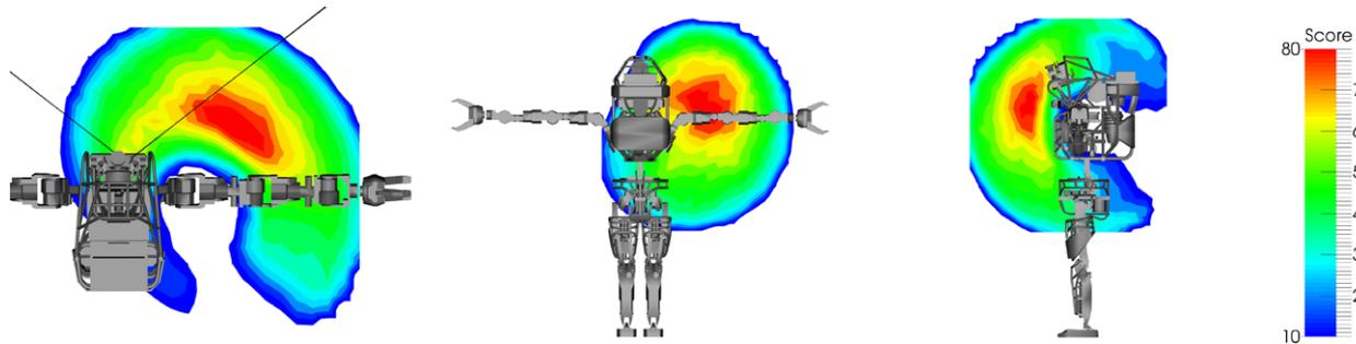
**Figure 2.** Visualization of the kinematic reachability of the robot from inferior (left), anterior (center), and medial (right) perspectives. We uniformly sampled 15 angles in the feasible range of each of the six right arm joints, divided the reachable workspace into  $20 \times 20 \times 20$  bins, and assigned each bin a score based on how many distinct end effector orientations it contained.
