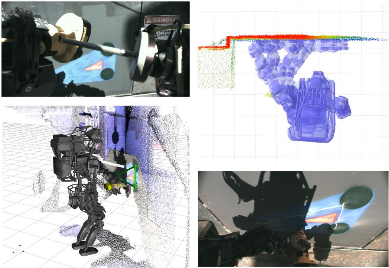
**Figure 16.** Top left: head camera view of the poker used to press the drill’s power button. Top right: visualization of the nominal plan to reach all drill target points in the triangle. Bottom right: head camera view provides situational awareness to the operator as the robot executes the drilling plan. Bottom left: Robot avatar and RGB point cloud visualization with affordance models of the drill and triangle target.
