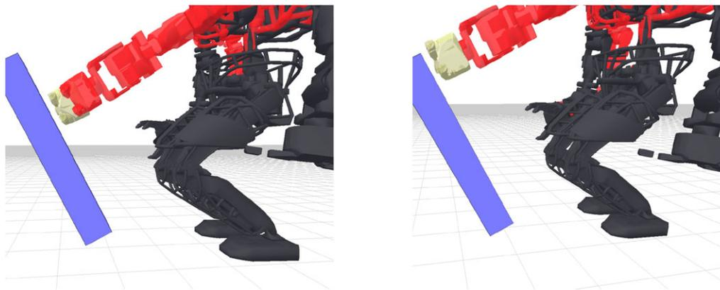
**Figure 9.** Relaxation of reaching plans to the affordance (blue) by the robot (gray). Left: a pregrasp reaching goal (yellow) just reachable (red) after automatic relaxation in position and orientation (by 2 cm and 3 degrees, respectively, in this case). Right: if the operator was unhappy with the relaxation, the reaching goal could be manually repositioned until precisely reachable. Here the planner is simultaneously solving for the six joints of the arm and the three back joints.
