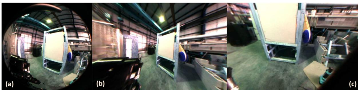
**Figure 4.** Fisheye lens rectification. (a) Raw image from the left chest camera exhibits severe fish-eye distortion and is difficult to interpret at the periphery. (b,c) After lens calibration, images can be rectified to produce arbitrary virtual viewpoints with minimal distortion.
