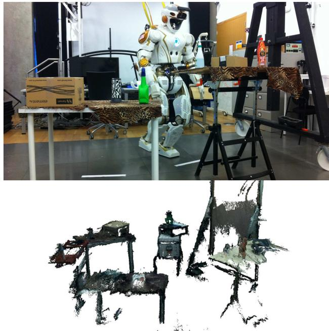
Fig. 1: Top: The NASA Valkyrie humanoid robot during operation in a laboratory environment. Bottom: stereo 3D reconstruction of a manipulation scene covering a 12m<sup>2</sup> area
