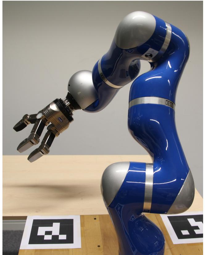
Fig. 5: KUKA LWR 4 (7DOF) with Schunk SDH2 (7DOF) mounted on table with AprilTags for camera pose estimation.
