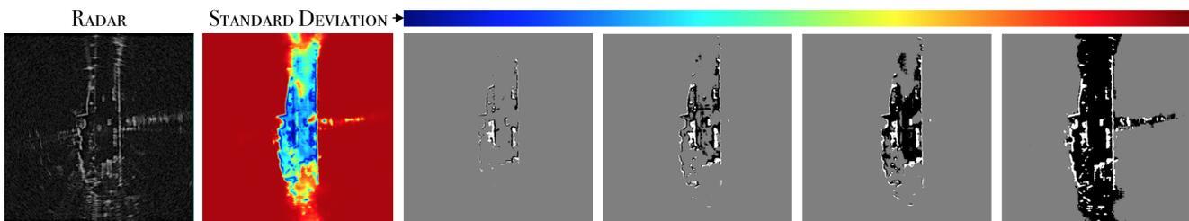
(d) A scene segmented as predicted occupied (white), unoccupied (black) and unknown (grey) for decreasing confidence thresholds (left to right) on the predicted standard deviation  $\gamma_\phi$ . From most certain to most least certain, we move from high power returns labelled as occupied, to a region nearby and up to the first return, to space that lies in partial and full occlusion.
