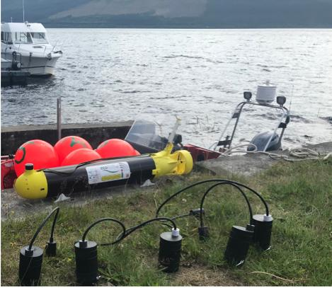
Fig. 1. ecoSUB AUV alongside 5 smart sensor nodes (foreground) at the trial site, Loch Ness, Scotland.
