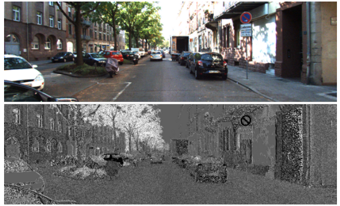
Fig. 4. Noise introduced by the lighting invariant transform in the KITTI dataset. The wide field of view results in many pixels with a single dominant RGB channel caused by the Bayer encoding across neighbouring pixels. As can be seen in Eq. 1, relatively small or large values in any channel will be amplified in the resultant transform.
