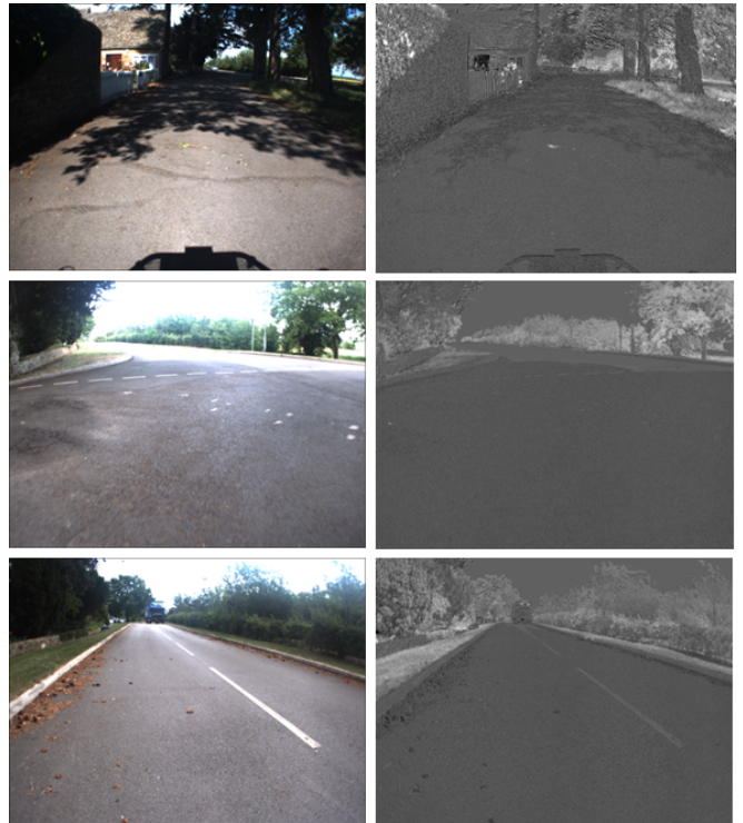
Fig. 3. Example lighting invariant images from the Oxford dataset. Shadows become less dominant in the images and the saliency of the material properties in the scene are increased.
