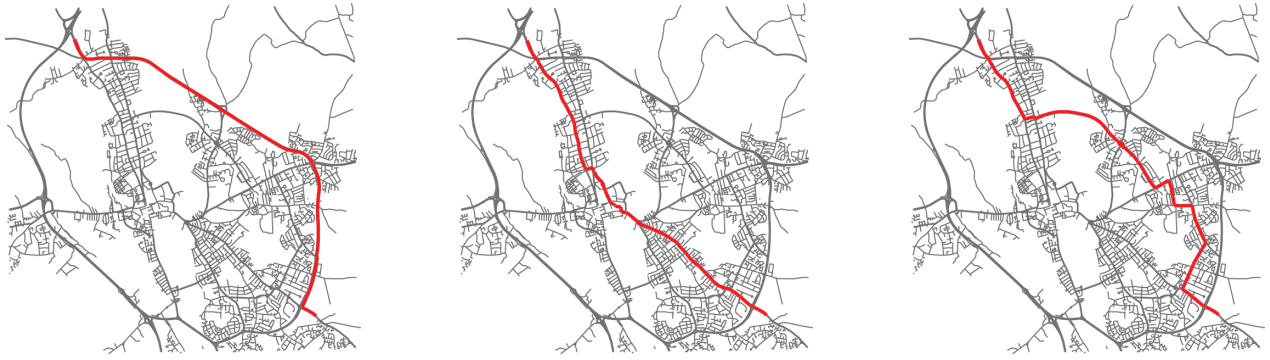
Figure 3: Examples of most likely trajectories between the same start and destination induced by three different route preferences. [left] minimum time traveled (the trajectory mainly follows motorways), [middle] minimum distance traveled and [right] custom preference learned from observations.
