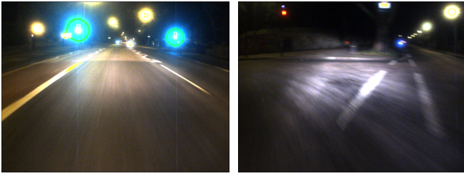
Fig. 2. Examples of scenes where point feature based methods fail. This is due to significant motion blur, saturation, lens flaring, and lack of well defined edges. In our approach we explicitly take advantage of the clearly visible light sources.
