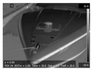
Figure 6: Boat surface reflection
