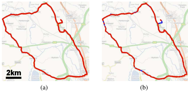
Figure 8: Loop closure maps for the 70 km dataset. Sections of the trajectory where loop closures exist are shown in red. (a) The ground truth. (b) Detected loop closures using FAB-MAP (100k CL), at 100% precision. The recall rate is 48.4%. A total of 2,300 loop closures are detected, with no false positives.
