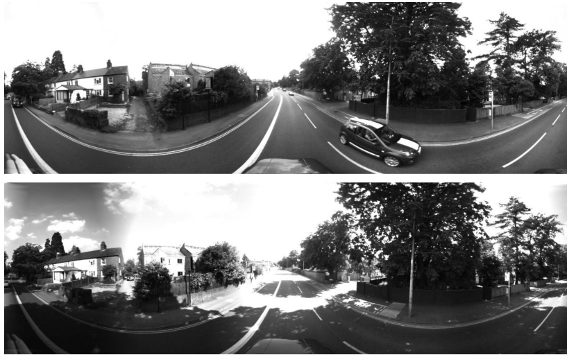
Figure 10: A correct loop closure from the 70 km data set. This is not an unusual match – the system typically finds correct matches in the presence of considerable scene change when the image content is distinctive.
