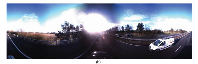
**Fig. 19.** The two highest confidence false positives in the 1000 km data set. Both matches are assigned probabilities very close to 1. In (a), we pass a similar-looking roundabout. The locations are 1 km apart. In (b), we encounter the same van twice. The locations are 9 km apart. Such rare-but-repetitive objects represent the most challenging class of perceptual aliasing.
