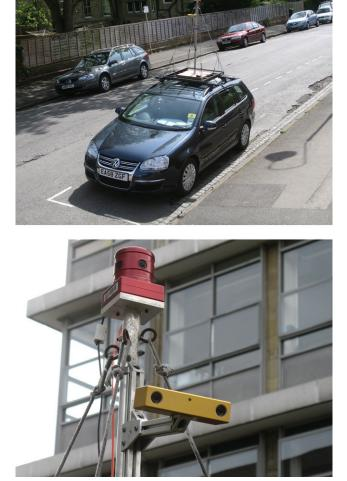
**Fig. 8.** Vehicle and sensor rig used to capture the 70 km and 1000 km data sets. The rig consists of a Ladybug2 omnidirectional camera and Bumblebee stereo camera, both from Point Grey Research. The cameras were mounted approximately 3 m above the road surface. GPS data was collected with a Seres unit from CSI Wireless, mounted on the roof of the car.
