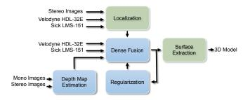
Fig. 2. An overview of our software pipeline. Our Dense Fusion module accepts range data from either laser sensors or depth maps created from mono or stereo cameras. We regularise the model in 3D space, extract the surface, and then provide the final 3D model to other components on our autonomous robotics platform (e.g., segmentation, localisation, planning, or visualisation). Blue modules are discussed in further detail in Sections III-IV.
