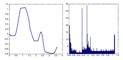
Fig. 5. The cumulative angular function is transformed into a histogram of angular values. Each bin contains the number of points along the cumulative angular function that have angular values that fall within the bin value. Using this histogram of bin values, the entropy of the cumulative angular function can be calculated.
