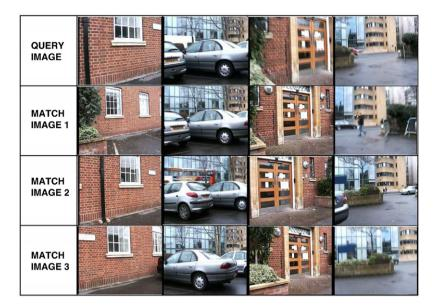
Fig. 9. Experimental results from our image query system. The top row contains the query images. Down the column are the corresponding matches in descending order of similarity. Notice the robustness of our image matching system against dynamic objects such as human and moving vehicles. However, the image in row 2, column 1 is an example of how visual match alone will produce wrong loop detection in environments where there are repetitive visual artifacts.
