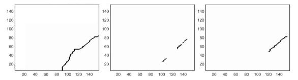
Fig. 12. From left to right: Sequence detection in visual similarity matrix, spatial similarity matrix and combined similarity matrix. The dark lines represents sequences of matching pairs of signatures.
