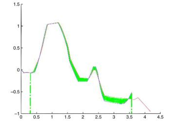
Fig. 7. Fig. 7 shows the disparity between two CAFs of two segments, S and S'. CAF is the one-dimensional representation of 2-D segments, which encodes the structure of the points within the segment by the change in tangential angles between consecutive points. The difference between the two CAFs is the area between the two curves. Segments that are similar to each other will have similar angular functions and correspondingly, the disparity between the two angular functions will be small.
