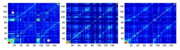
Fig. 11. Similarity matrices. The left matrix is the image similarity matrix. The middle matrix is the laser scan similarity matrix. The right matrix is the combined image–laser scan pair similarity matrix. Improvement in loop closure detection can be observed by the improved definition of the off-diagonals of the combined image and laser scan pair similarity matrix over the off-diagonals of the other similarity matrices.
