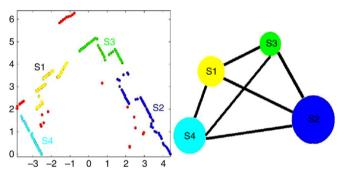
Fig. 4. This shows a typical geometry patch after segmentation and a graph depiction of the way we encapsulate the information contained. Each node is a segment and contains the CAF function, its entropy measure and a list of critical points. The edges represent a known spatial relationship between segments.
