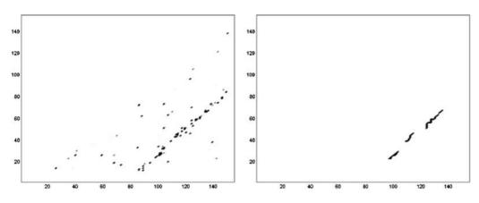
*Figure 33.* On the left is a lower triangular matrix of a spatial similarity matrix (SSM) after loop closure has occurred. On the right is the result of applying the sequence extraction algorithm.
