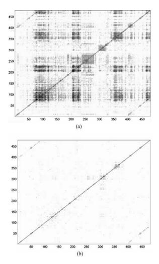
*Figure 6.* (a) shows a visual similarity matrix constructed from images collected from an exploration run (around the path shown in Fig. 17). (b) shows the visual similarity matrix after rank reduction. Note that the off-diagonal dark line (which signifies the true loop closure) has not been affected by the rank reduction whereas visually ambiguous regions within the similarity matrix have been removed.
