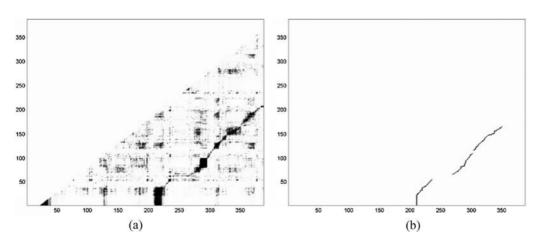
*Figure 4.* (a) A lower triangular matrix of a visual similarity matrix after loop closure has occurred. (b) The result of applying the modified Smith-Waterman algorithm to find significant local alignments.
