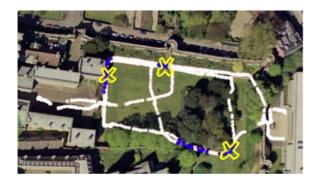
*Figure 18.* An aerial image of the test scenario—New College Gardens. The position of the mobile robot is measured by a GPS receiver with positional uncertainty of around 5m. The path taken by a mobile robot is marked with white crosses. There are various breaks in GPS signal reception. The large yellow crosses mark the positions where loop closure is detected.
