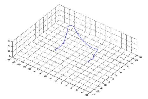
*Figure 15.* The pre-loop closing estimated trajectory of the vehicle. The sharp turn compounded with long gently curved traversals leads to a gross error in position estimate. Each cell is 20 by 20 m.
