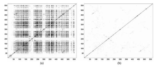
*Figure 19.* (a) shows the highly ambiguous visual similarity matrix constructed from images from the "New College" data set. (b) shows the visual similarity matrix after rank reduction. Note that the off-diagonal dark line (which signifies the loop closure) has not been affected by the rank reduction whereas visually ambiguous regions within the similarity matrix have been removed. Due to multiple loop closure at different locations, there are multiple dark off-diagonals.
