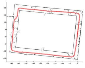
*Figure 31.* A post loop closure 2D SLAM map of the cloister with robot trajectory. The map is built with a 2D laser scanner and the southern, east-west traversal is as shown in Fig. 26. The curved structures appearing to cross the cloister corridors are artifacts stemming from the uneven floor pitching the vehicle and causing the laser scans tp intersect the floor before the walls.
