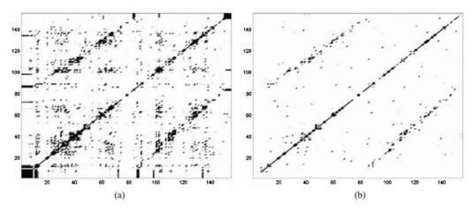
*Figure 32.* (a) shows a spatial similarity matrix (SSM) constructed from laser scans collected from an exploration run around a building. (b) shows the similarity matrix after rank reduction.
