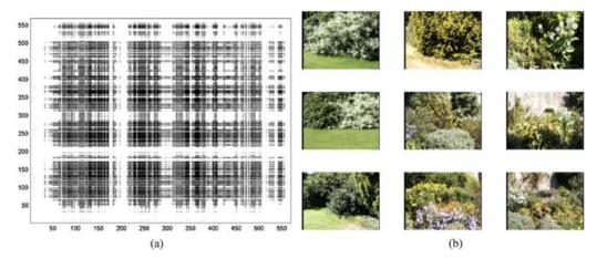
*Figure 20.* (a) shows the first rank one approximation of the visual similarity matrix shown in Fig. 19. (b) shows nine images with the highest scores in  $v_1\lambda_1v_1^T$ . These images are mostly images of vegetation.
