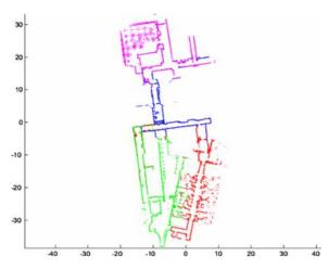
*Figure 40.* A fused map formed by detecting intersections between and aligning the four local maps shown in Fig. 37.
