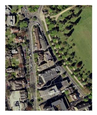
*Figure 17.* An aerial image of the workspace with the final estimated vehicle trajectory and metric grid superimposed upon it.
