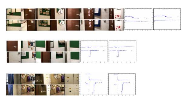
*Figure 39.* Matching subsequences between image streams gathered by different robots. The local regions in each map are shown to the right of each pairing—the first for the top sequence and the second (far right) for the second (lower) sequence.
