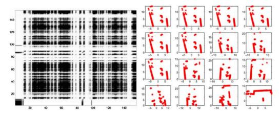
*Figure 35.* On the left is the  $v_2 \lambda_2 v_2^T$  approximation of the spatial similarity matrix shown in Fig. 32. On the right are 16 laser scans with the highest scores in the matrix. These laser scans can be broadly defined as having parallel lines.
