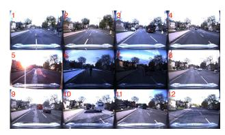
Figure 7. Camera images from a sample location for all twelve evaluation datasets. The traversals include significant variation in lighting and weather, including direct sunlight in dataset 5, snow in dataset 6 and seasonal vegetation change in dataset 9. Dataset 1 is used to build the scene prior; all subsequent datasets are matched to dataset 1.
