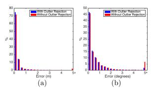
Figure 8. Error histograms for translation (a) and rotation (b) for all datasets combined. 94.5% of translational errors were under one metre in magnitude, and 79% of rotational errors were under one degree. Outlier rejection successfully removed the vast majority of errors over 5m or 5°.
