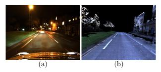
Figure 12. Failed localisation between a night-time dataset (a) and daytime prior (b). The localisation failed to converge for all images collected at night, due to the highly non-uniform illumination. A possible solution is a separate appearance prior collected at night, but this doubles storage requirements.
