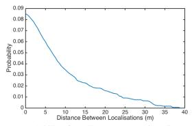
Figure 9. Probability of travelling more than a given distance without a successful localisation. The likelihood of travelling more than 10m without localisations (using odometry alone) is less than 3%.
