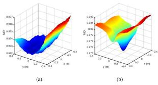
Figure 5. NID cost surface for the calibration transform  $G_{LC}$  in x and y axes for (a) one image and (b) ten images. With a single image the cost surface is rough and contains multiple minima, depending on the local structure. By optimising over multiple locations simultaneously, the cost surface is smoother and contains a distinct single minima. The effect is similar for the other four axes.
