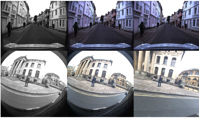
Fig. 9. Left-to-right: raw Bayer image (provided in PNG format), demosaiced colour image, and rectified perspective image from (top) Bumblebee XB3 and (bottom) Grasshopper2 cameras. MATLAB functions for demosaicing and undistortion are provided in the development tools.
