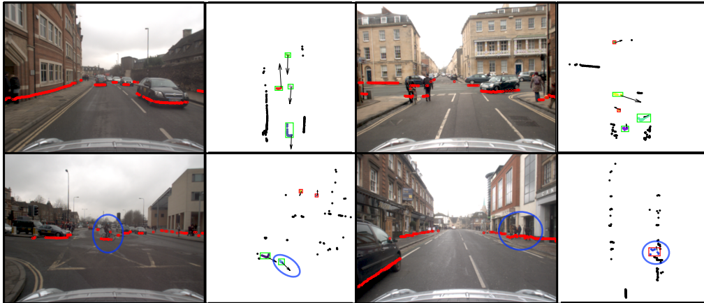
Figure 5.8: Examples of cases where the proposed system is able to successfully detect and track dynamic objects under challenging situations. As in Figure 5.1, green boxes represent true detections according to the ground truth labels, and red boxes denote false alarms. Blue ellipses highlight interesting situations in the scene. Images are provided for visualisation only . See text for details.
