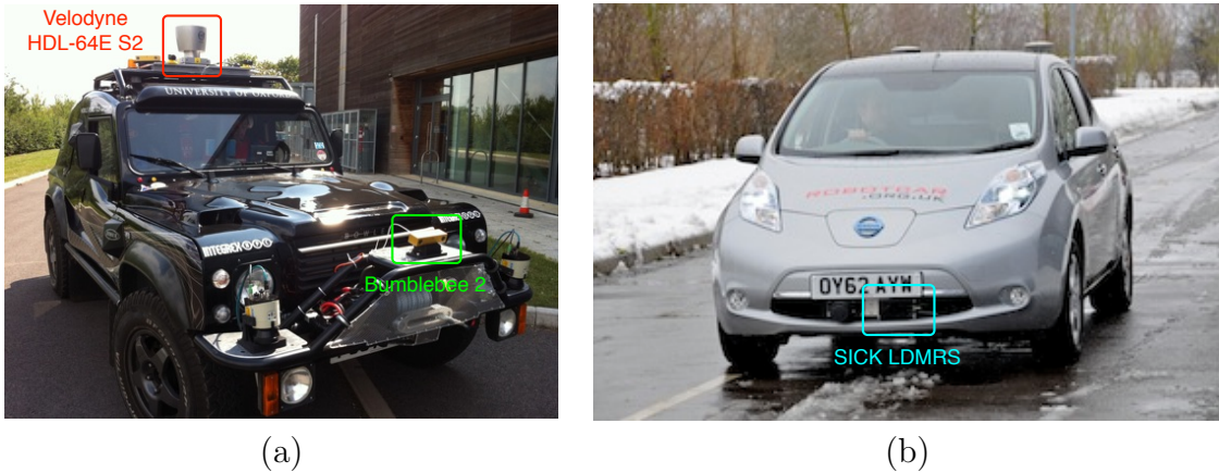
Figure 1.1: Our research platforms deployed in this thesis. (a) The Bowler Wildcat research platform, equipped with a Velodyne HDL-64E S2 3D scanner (highlighted in red), and a Bumblebee 2 stereo camera (highlighted in green). (b) The RobotCar autonomous driving platform equipped with a SICK LDMRS laser range finder (highlighted in cyan).
