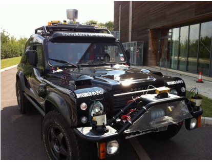
Fig. 3. The Bowler Wildcat research mobile platform, equipped (on top) with a Velodyne HDL-64E S2 sensor.
