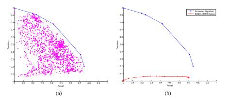
**Fig. 3** (a) Scatter plot of the obtained 1803 sample parameter settings using [10] with the estimated frontier overlaid. (b) Precision-Recall tuning curves for the proposed system and the SICK LDMRS native tracking system.
