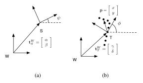
**Fig. 2** Illustrations of frame conventions and variable definitions. (a) Transform from the sensor frame to the world frame. (b) Transform from a track frame to the world frame, with boundary points represented locally to the track frame.
