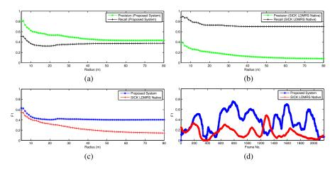
**Fig. 4** (a) Precision and Recall versus operating radius for the proposed system. (b) Precision and Recall versus operating radius for the SICK LDMRS's native system. (c)  $F_1$ -measure versus operating radius for both systems. (d)  $F_1$ -measure over past 100 frames versus frame number for both systems.
