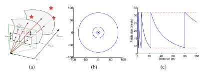
Figure 3: True scale distance rings. (a) A fixed 3-D region size between distances  $d_{min}$  and  $d_{max}$  projects to template sizes ranging from  $s_{max}$  to  $s_{min}$  with size in  $\frac{1}{d}$ . For  $d > d_{max}$ , a bigger fixed 3-D size can be computed to provide image templates within the same pixel size range. (b) This figure illustrates the different bands for true scale computation that become bigger with distance. (c) Patch sizes according to distance.
