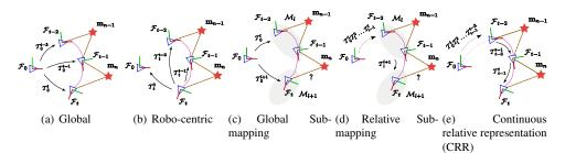
Figure 1: Different pose and landmark representations with  $\mathbf{m}$  for landmarks,  $\mathbf{F}$  for frames,  $\mathbf{T}$  for transforms and  $\mathbf{M}$  for sub-maps where applicable. Dashed lines represent measurements. Landmarks are connected to their base frames by filled lines. '?' indicates the difficulty in sharing information between sub-maps.
