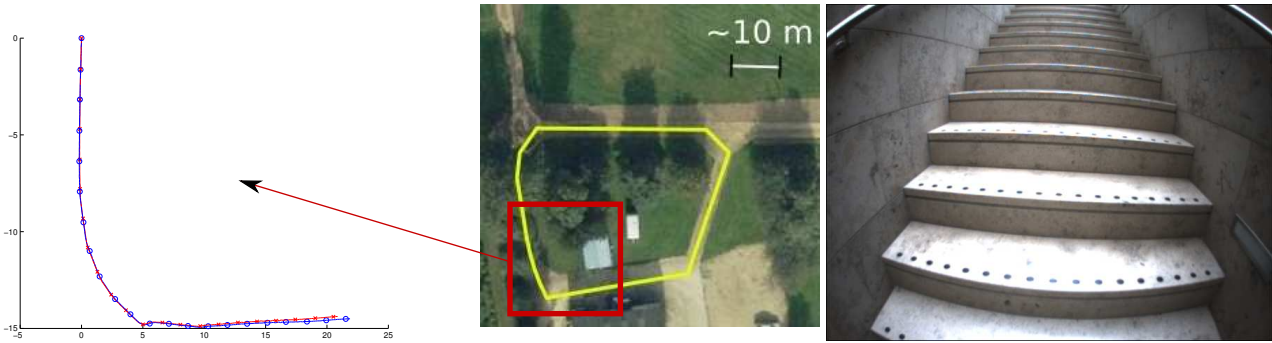
(a) Comparison of the trajectories produced by PTAM and RSLAM on the longest continuous set of frames tracked by PTAM on the Begbroke sequence. It is comprised of around 800 frames or about 40m. The trajectory estimated by PTAM is in blue with circles and the one estimated by RSLAM is in red with crosses. The accuracy was similar for both systems.
