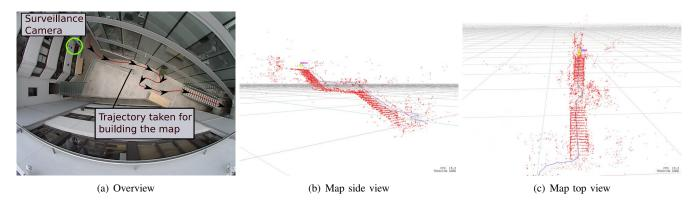
Fig. 7. An indoor sequence was used to test the system. (a) shows a top view of the scene with the surveillance camera and the trajectory taken to build the map. (b) and (c) show the estimated trajectory and map. The structure of the steps are apparent. The first floor appears parallel to the ground and the staircase are aligned indicating that the pose and map are correctly estimated.
