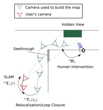
Fig. 1. The user's camera cannot see the hidden view so we require an indirect way of computing its position with respect to the surveillance camera. The idea proposed in this article is to build a map beforehand and register one of its views with the surveillance camera (this gives us  ${}^{s}\mathbf{H}_{o}$ ). At run-time, the system relocalises with the map (this provides  ${}^{n}\mathbf{H}_{o}$ ) and can then transfer the hidden view live to the camera.
