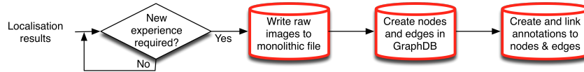
Fig. 9 Overview of the EBN experience creation pipeline. This process has less strict runtime requirements and runs in a background thread. Writes to the database are highlighted in red.
