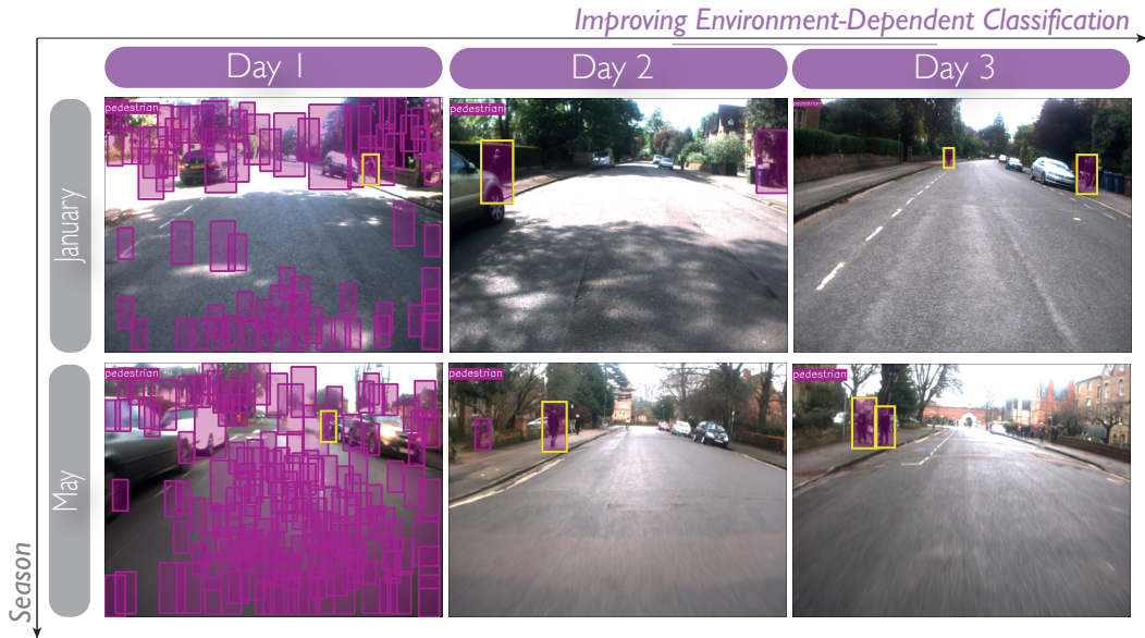
Figure 1: Images from a route in Oxford at two different times (January and May) on which we performed pedestrian detection. We demonstrate a great improvement in performance over a few EBC iterations by automatically adapting the detector to different seasons. False positives are shown in purple, while true positives have a yellow bounding box. Figure best viewed in colour.
