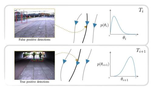
**Fig. 2.** Overview of proposed method. A new traversal (black line) of a route that has been traveled previously (gray lines) can make use of past estimates of detection performance. For instance, at Location A where we have repeatedly observed false positive detections, the performance record yields a low probability of success for the detector, while at Location B, where the detector has only produced true positive detections, the probability of success is very high.
