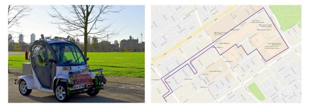
**Fig. 6.** Platform and route chosen for experiments. The vehicle is equipped with a Bumblebee3 stereo camera, Velodyne Lidar HDL32E, and an INS system for data collection. We produce both 2D and 3D pedestrian detections in image and laser data along the route in Milton Keynes, England, shown on the right.
