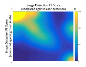
**Fig. 7.** Heatmap showing a strong correlation between performance scores for the SVM+ACF detector computed in two different ways. First, the 2D detection  $F_1$  score is computed using ground truth annotations (*y*-axis). Second, the same score is computed using laser detections instead of ground truth (*x*-axis). The diagonal elements, as well as the peaks at 1 and 0, allow us to believe that very little noise will be introduced by using a surrogate metric of performance.
