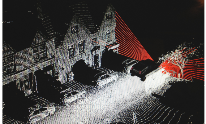
Fig. 1. An example of a swathe which can be thought of as a 3D point cloud built up as a push-broom 2D LIDAR sweeps through an environment with vehicle motion. The red lines illustrate the latest scan from the 2D LIDAR, which is mounted on the front of our Bowler WildCat research platform. This swathe was constructed using calibration estimates obtained from the proposed method relative to a stereo camera providing a trajectory derived from visual odometry.
