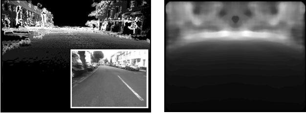
(a) Representative Jacobian image given by Equation (6) (i.e., evaluating \partial z^s / \partial \mathbf{x} for each pixel). Camera image provided for reference.
