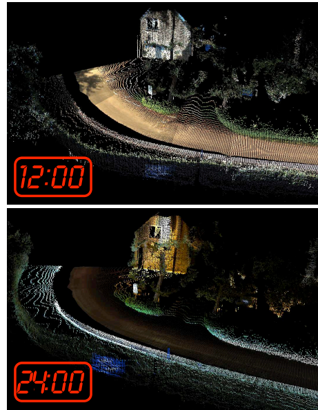
Fig. 7. Sample sections from the coloured 3D point cloud scene priors built using the midday and midnight datasets for the same physical location, showing the dramatic change in the appearance of the scene between day and night. The blue-white streaks in the verges off the road in the midnight prior are due to the LEAF’s headlights, and the orange orb at the top of the building is a streetlight. Note that although the pointcloud is coloured here with RGB for ease of presentation, we store both RGB and illumination invariant appearances for each point.
